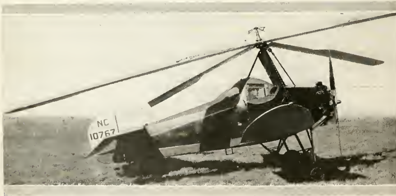
The new American Kellett autogiro with removable cabin enclosure for winter flying
